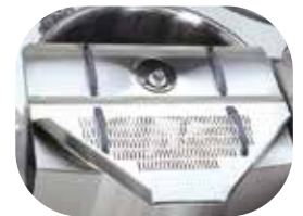
Strainer plate extension for 300-400 litre kettles
