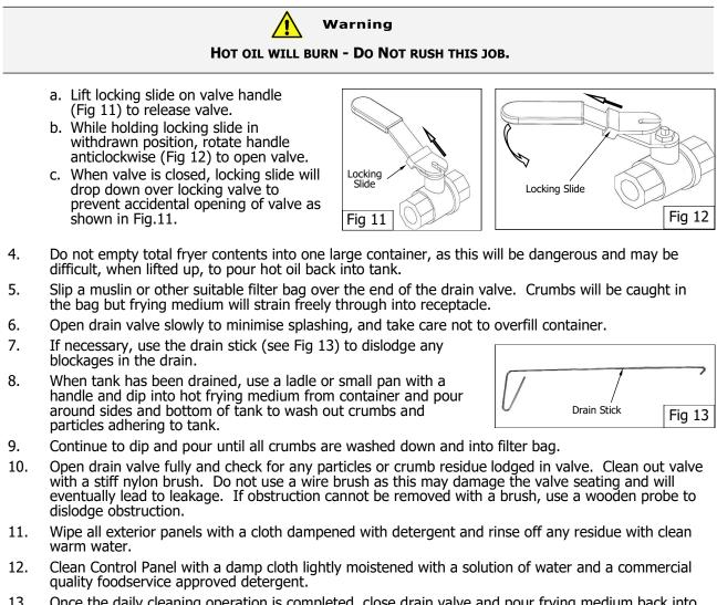
13. Once the daily cleaning operation is completed, close drain valve and pour frying medium back into tank.
