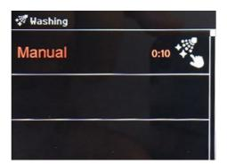
The display reads "Cool" if the chamber temperature is too high, "Wait" if the chamber temperature is too low. When the temperature is reached, the message "Insert detergent" will appear, an acoustic signal will notify that it is time to open the door and spray the detergent into the cooking chamber.
