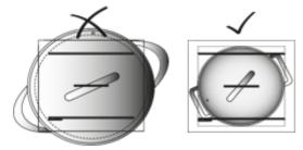
• Pans must fit the glass! The best pan to use is the one with a bottom that fits the coil.
