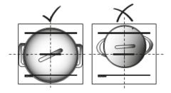
• The pan must not cover more than one cook zone on dual, twin dual or quad units.
