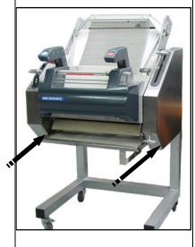
**3.** Unhook and tilt back the Lightspeed Guard Mouth assembly to allow access to the rollers.
