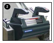
**4.** Open the rear and front sheeting rollers to max open position.
