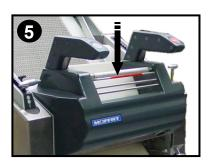
The moulder must **stop** operating immediately. If the machine does not stop, do not use.
