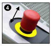
The moulder must **stop** operating immediately. If the machine does not stop, do not use. Call supervisor and advise Moffat service agent.
