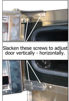
Slacken these screws to adjust door vertically - horizontally.
