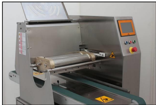
2. Delicately insert the two rollers
