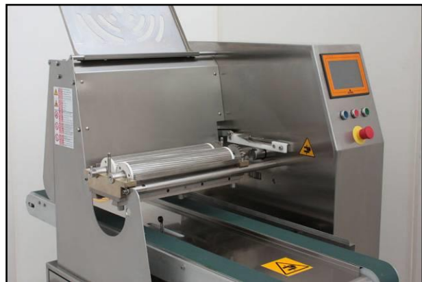
2. Delicately insert the two rollers
