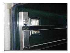
b. Wash the glass lens with a soft sponge using warm water and a detergent solution. Rinse with clean, warm water.
