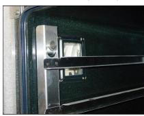
b. Wash the glass lens with a soft sponge using warm water and a detergent solution. Rinse with clean, warm water.
