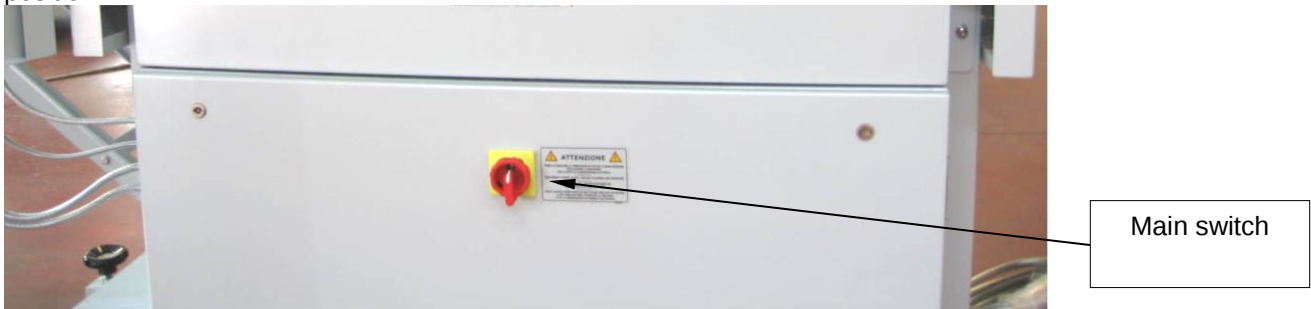
Figure 3 - Main power switch
