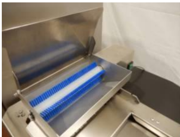
Figure 17 - Loaf moulder flour duster
