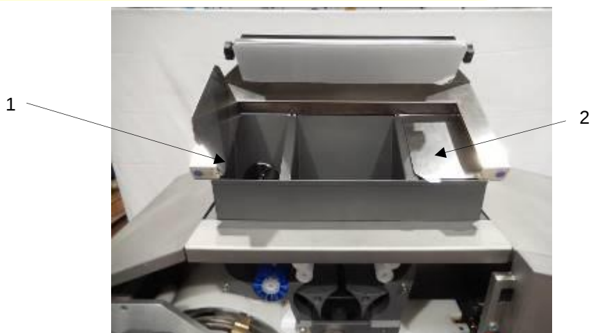
Figure 16 - Loading the flour in the two pockets on the sides of the hopper
