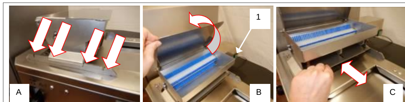
Figure 20 - Loaf moulder flour duster
