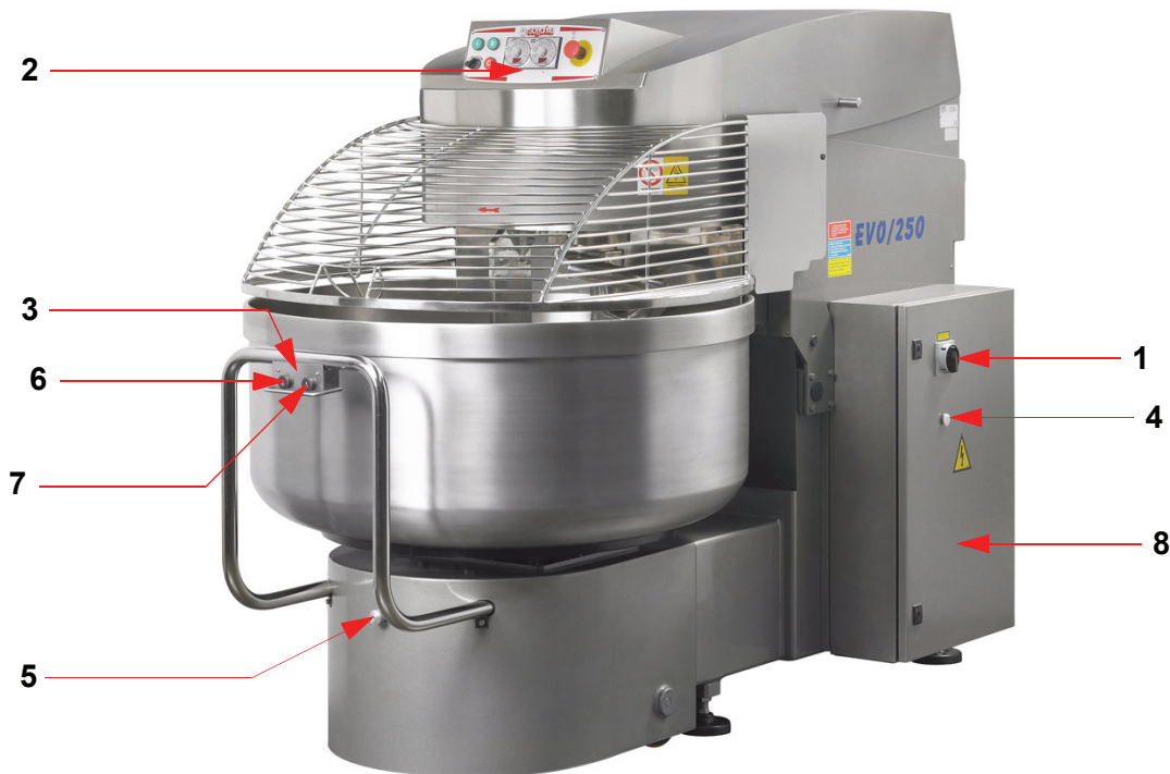
Fig. 11 Main switch and control panel
