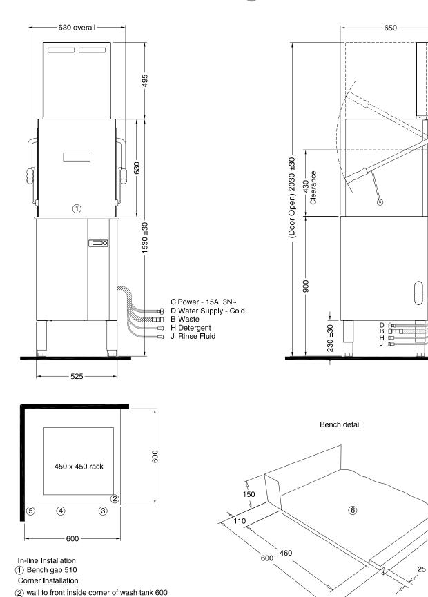
(3) machine must face left for access to controls
