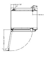
Model E31D4/2 shown Model E31D4/2C dimensions: Add 31/4" / 82mm to vertical heights
