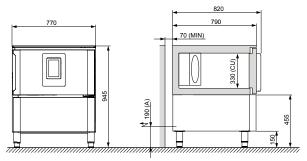
(A) Electrical power supply (CU) Useful (MIN) Minimum
