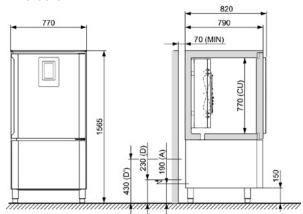
Electrical supply (SG) Without housed unit (D) Liquid line 3/8" (D') Suction line 5/8"
