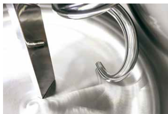
Straight Breaking Column
